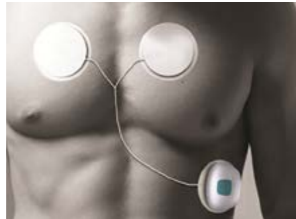
Zensor is a wearable monitoring device that detects heart arrhythmias.
